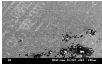
Fig. 5 SEM image of NiCr alloy in sodium fluoride
