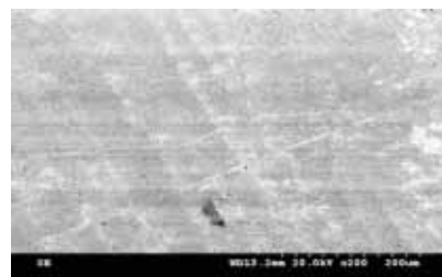
Fig.3 SEM image of NiCr alloy in artificial saliva
