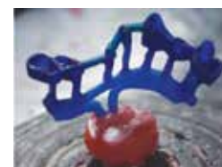
Fig. 6 Bar castable bar contoured to ridge and sprue attached
