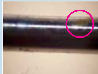
Fig. 10: Rust on the stainless steel wire dipped in concentrated salt water compared with the control
