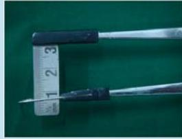
Fig. 2 Measuring tip consisting of scale and the stop
